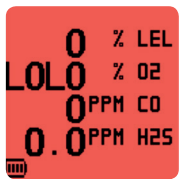
Red display in alarm conditions
